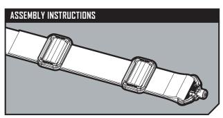
To connect the *QDM Sling Swivel* to the sling, run the end of the *MS1 Sling* through the *QDM Sling Swivel* and then back through the *Fit Buckle(s)*. Double the webbing back through the upper *Fit Buckle* if possible.
